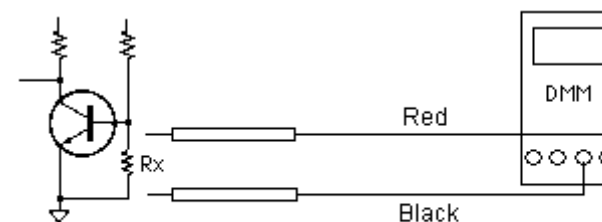
Rx is measured without the influence of transistor junction
